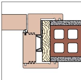
Finger-joint snap-fitting between casing and jamb, Pivato patented
