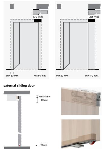
ILA, the sliding door, is a real "wall" in motion; its slide bar is hidden, when the door is opened, or when it is closed. Ideal for use as external sliding door, it can be a valuable addition to close walk-in closets or small opening equipped with shelves as bookcases or mini-bar.
